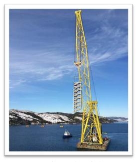
Heavy lift vessel (TakLift 6) at deep water site.
