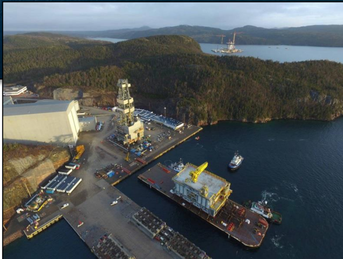
The Drilling Support Module (DSM) arriving at the Bull Arm quay from Marystown in December 2015. GBS at deepwater site visible in the distance.
